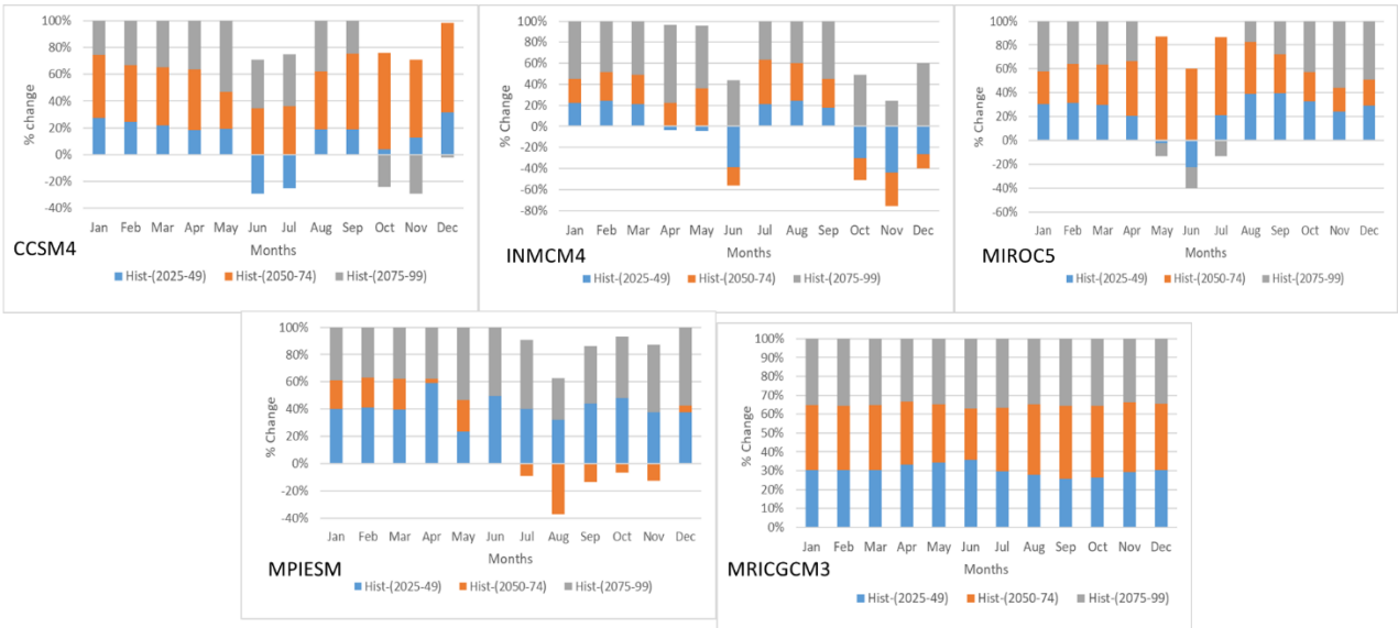
Fig.4.38: Percent change of discharge between different time periods under RCP4.5 for the condition of change in both climate and LULC
